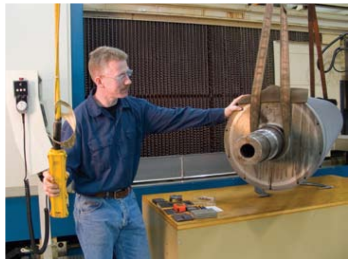
Easy does it! Doug Botten loads a 12,000 lb. monster – Twenty-four inches in diameter and solid except for a three inch diameter hollow through the center. Like every roll, it presents its own challenges in compensating for sag to achieve the desired linear profile.
