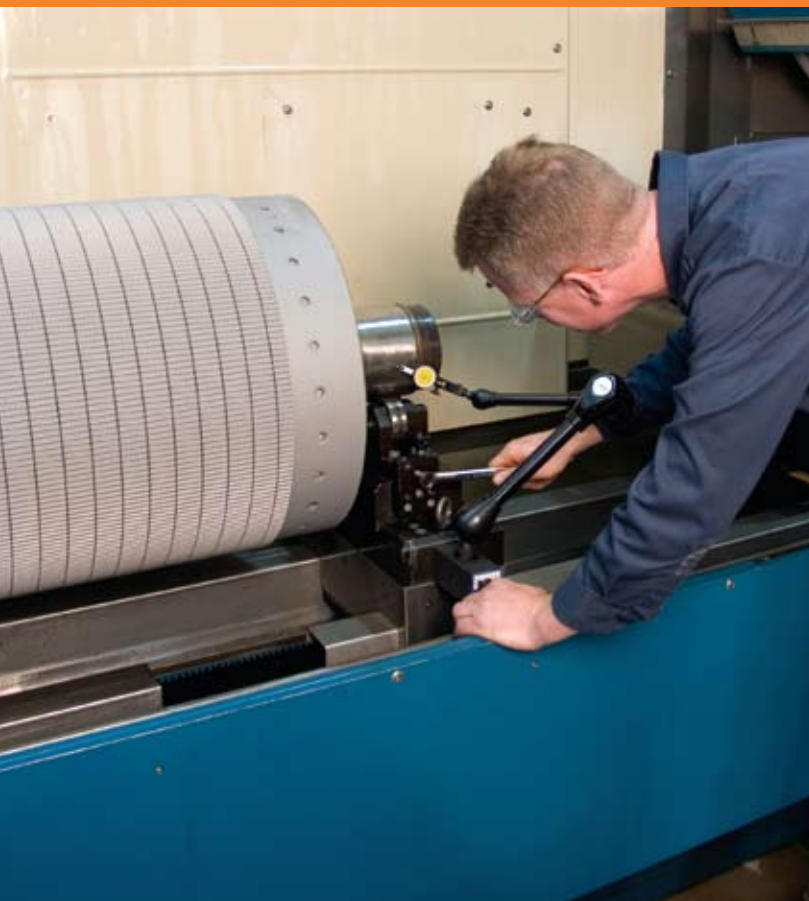
Top Left: Although the Mägerle has a probe to measure part position and calculates offsets, craftsman Doug prefers to measure it and make adjustments himself. Top Right: Mägerle MGC with a triple flute C-profile wheel grinding solid core at 31 inches/minute at full depth of cut with a stock removal of 0.15 inches deep.
